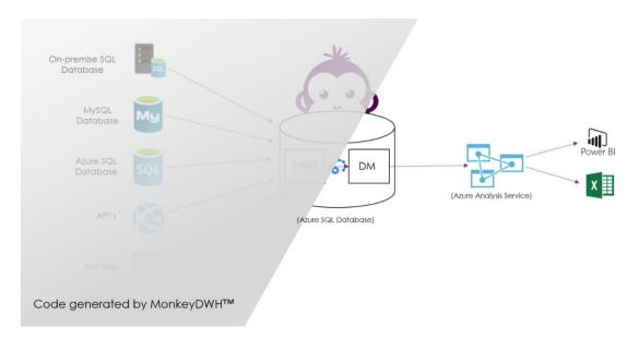
The MonkeyDWH<sup>™</sup> generates all Azure SQL database- and Data Factory objects needed to extract data from different kind of sources and store data historically inside the DWH. It also generate database tables for the DM and the required ADF pipelines and datasets.
